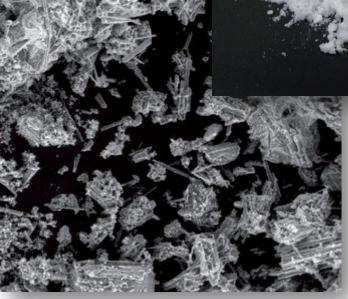
Magnesium ammonium phosphate hexahydrate: MgNH<sub>4</sub>PO<sub>4</sub>.6H<sub>2</sub>O
