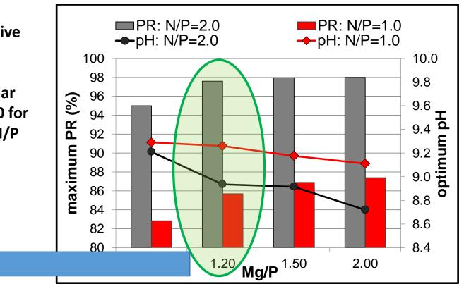
P-OP=200 ppm T=25°C Optimal pH operating conditions and maximum PR (%) at molar ratio Mg/P (1.0, 1.2, 1.5 and 2.0) and N/P (1.0, 2.0).
