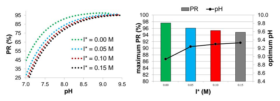
Effect of ionic strength in the optimal pH operating conditions and maximum PR (%) at molar ratios Mg/P = 1.2, N/P = 2.
