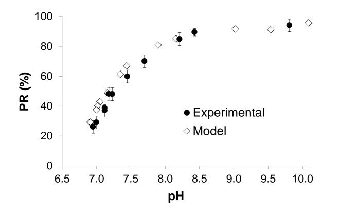
Predicting and measured PR (%) as struvite for P-OP =200 ppm at the molar ratios Mg/P=1 and N/P=2, T= $25^{\circ}$ C.
