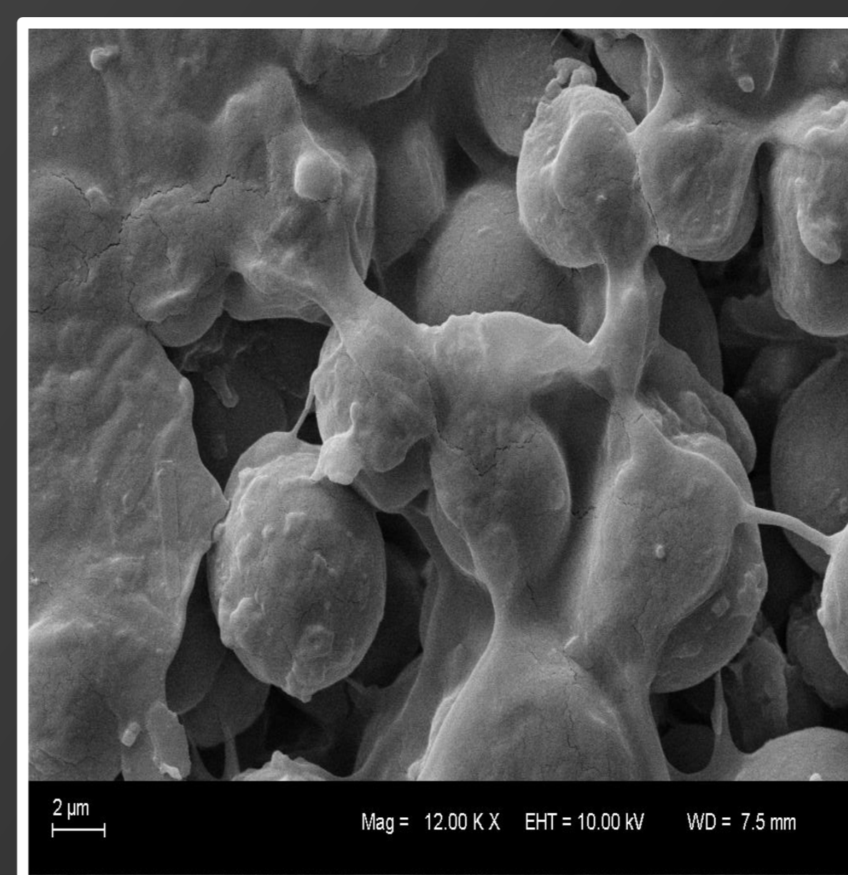
Fig. 2 Scanning electron microscopy (SEM) of pancreatic lipase immobilized on bleached coconut pulp with glutaraldehyde
