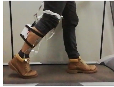
Fig. 2: Gait subphases detection tests. The picture depicts a participant walking on a treadmill with the H-GAIT NP.
