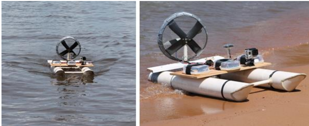
Figure 3. Testing of the ASV prototype
