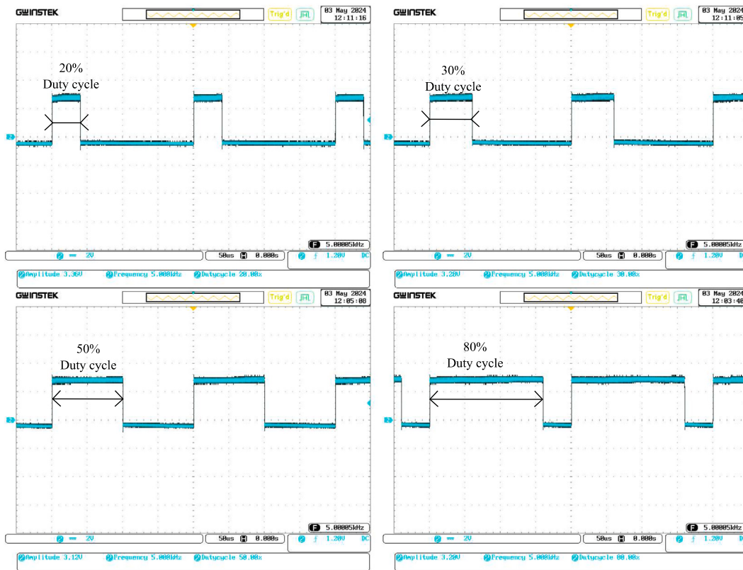
Fig. 9. The PWM observed with the oscilloscope.
