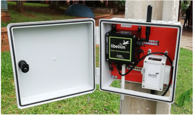
Fig. 2. Solar-powered air quality monitoring station based on the Libelium Smart Environment Pro platform, integrating an Alphasense OPC-N2 sensor for PM_{10} , PM_{2.5} , and PM_{10} measurements, a meteorological sensor, 4 G communication, and an IP65 weatherproof enclosure with autonomous power supply.
